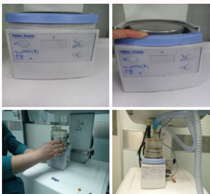
Figure 2: Connection of the ventilator humidification tank: one pressure; two pushes; three releases.
