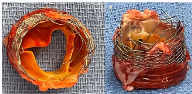
Figure 2: The extracted LOTUS Edge prosthesis, top (A), and (B) side views.
